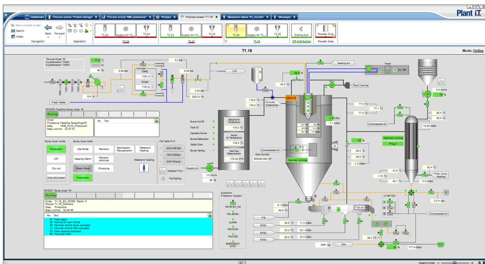
Process image of the dry section – one of three drying towers
